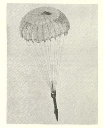
NEW PARACHUTE DESIGN for B61-3 has been undergoing testing at Sandia Laboratories. In this series of three photographs, the 24-foot-diameter parachute is subjected to a Mach 1.4 deployment and a load of 90,000 pounds at Sandia's rocket sled facility. New material, Kevlar-29, is used in the chute. The project is centered in Parachute Systems Division 1332 under Dave McVey.
